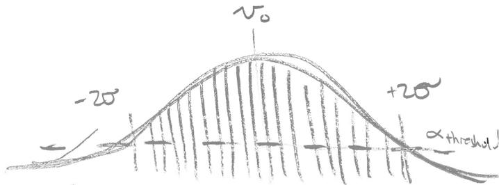
So between  $-2\sigma$  and  $+2\sigma$  on our gain curve, we can achieve lasing. That freq. span,  $4 \times 10^{12} \text{ Hz}$ , supports  $\frac{4 \times 10^{12} \text{ Hz}}{10^{10} \text{ Hz}} = 400$  modes.
